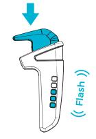
When the remote successfully pairs with the board, all five LEDs will flash once.
