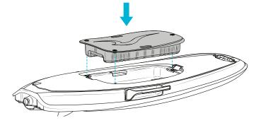
Locate the three spring-operated button holes.
