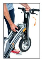
Bring the fork close to the frame until you hear the CLICK, which locks the mechanism.
